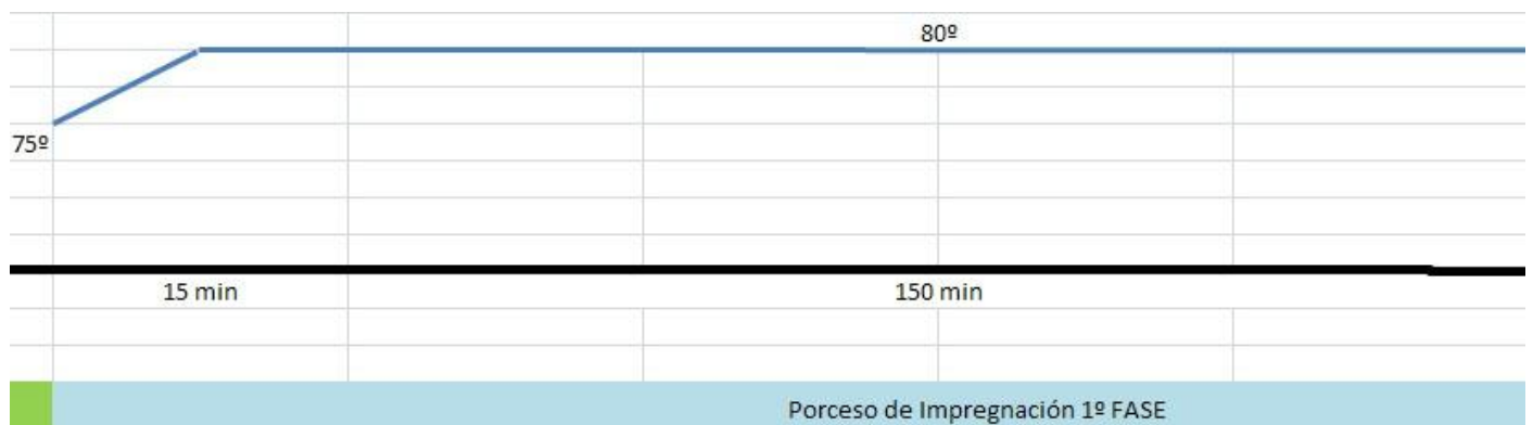
Graphic 2 Drying process 1 st stage
