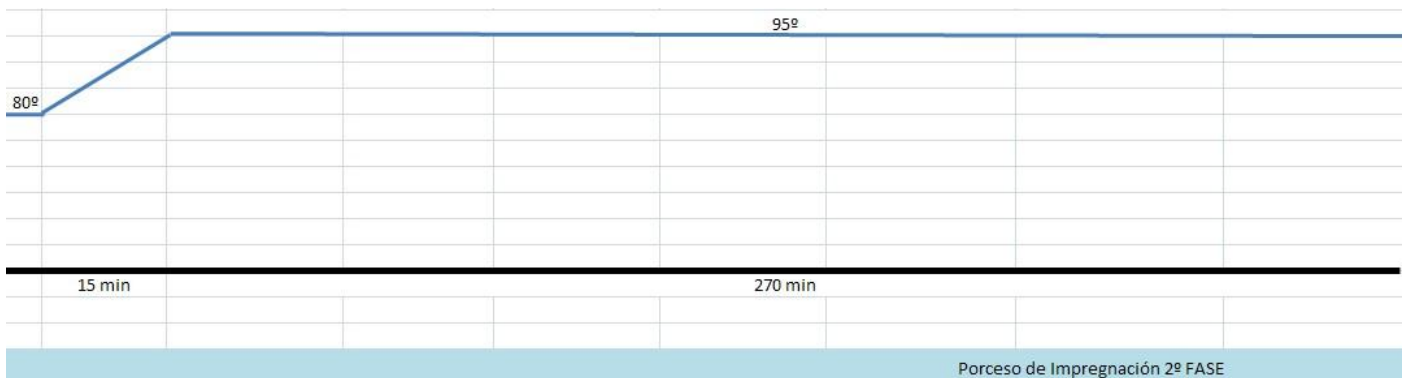
Graphic 3 Drying process 2 st stage
